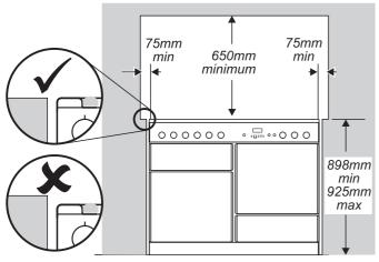
The hotplate surround should be level with, or above, any adjacent work surface. Above hotplate level a gap of 75mm should be left between each side of the cooker and any adjacent vertical surface.
